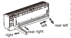
When select leading out the pipe from left or right, please cut off the corresponding hole on the bottom case.
