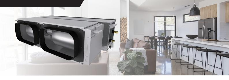
The new PEA-M HAA Ducted unit has a two-piece construction<sup>\*1</sup>. This allows separation of the indoor unit heat exchanger and fan deck assembly for easier handling and installation into the roof space.
