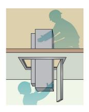
Easier Installation The fan deck section and the heat exchanger can be separately transported and assembled in the ceiling space.\*<sup>3</sup>
