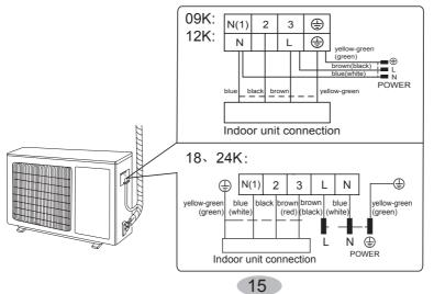
2. Fix the power connection wire and signal control wire with wire clip (only for cooling and heating unit).
