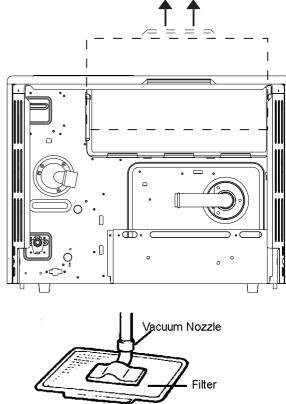
Ensure to fit the Fan Filter back in the appliance after cleaning. DO NOT operate appliance without filter in place.
