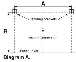
9. Attach the two securing brackets supplied to the wall using the two 8g x 30mm screws supplied, or suitable equivalent refer to diagram A.
