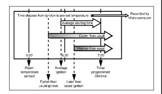
The temperature differential at the time of sensing the room temperature combined with the data from previous operation governs exactly how long before the programmed 'ON' time the micro-computer will operate the heater and ignite the burner.
